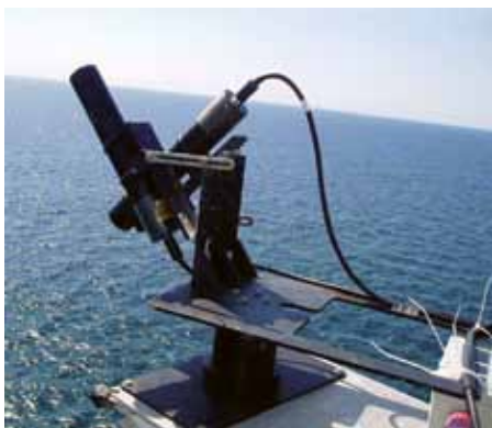
FIGURE 8 Satlantic SAS hyperspectral radiometer, mounted on vessel superstructure
